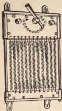
FIG. 52.—Common type of resistance frame. By moving the lever on the row of studs, one or more of the coils of iron, German silver, or other high-resistance metal, may be thrown into circuit; thus varying the line resistance at will.
